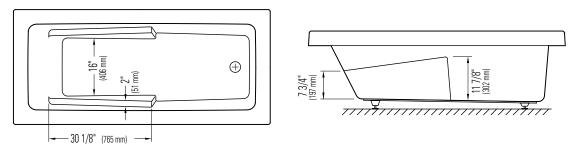
\*A bathtub fitted with back jets can cause the pump to protrude by approximately 3" from the overall dimension.
