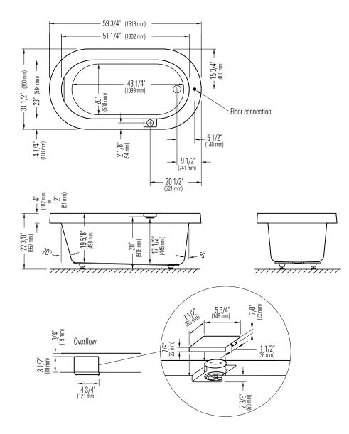
\*A bathtub fitted with back jets can cause the pump to protrude by approximately  $3^{\prime\prime}$  from the overall dimension.
